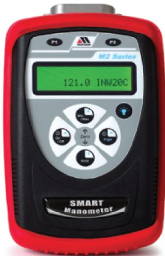
This precision, handheld, digital pressure reference manometer allows for convenient calibration of pressure transducers. The M2 series can be recalibrated in the field for zero, span, and linearity. The user has the option to select a 1 point or 5 point calibration procedure. The manometer enables users with accurate primary standards to calibrate their devices locally if desired.
