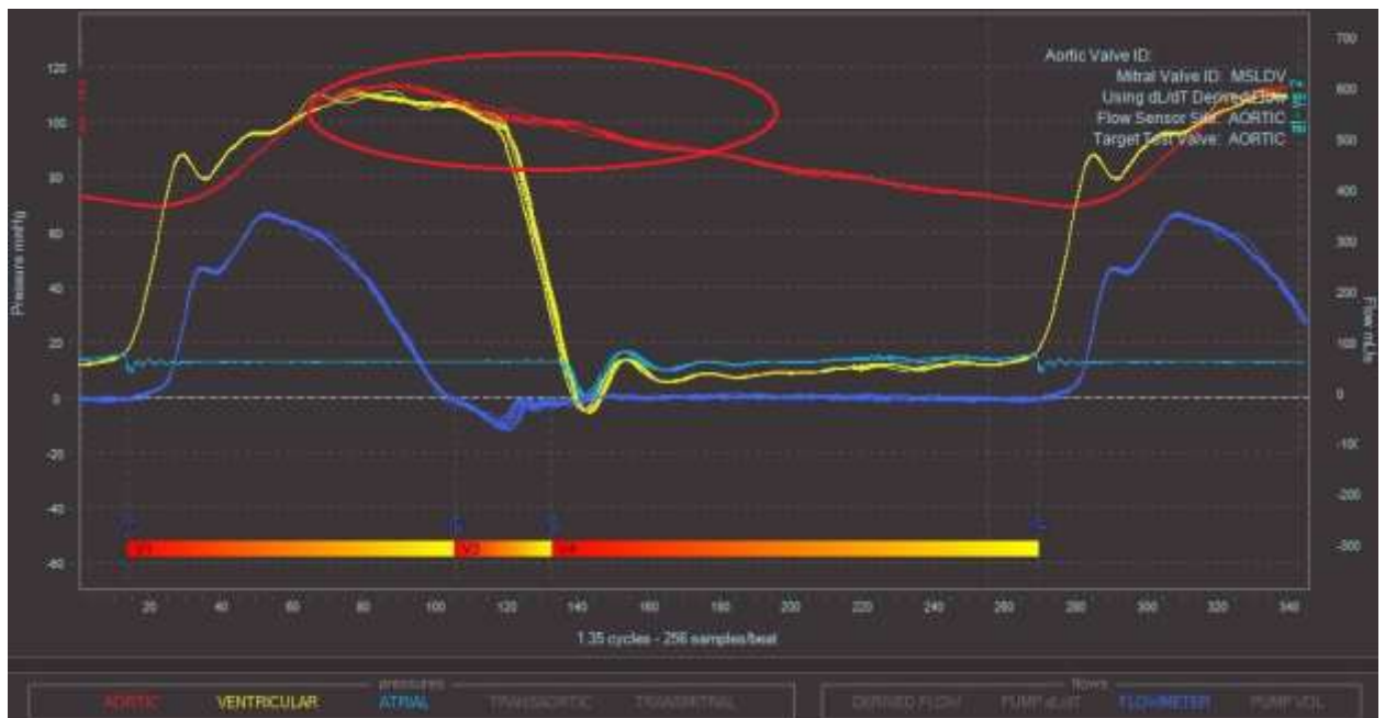
Aortic pressure (red) noise due to improper Aortic Root Compliance pressurization.
