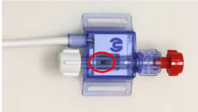
Bubbles may be trapped at the pressure transducer crystal if not flushed properly.
