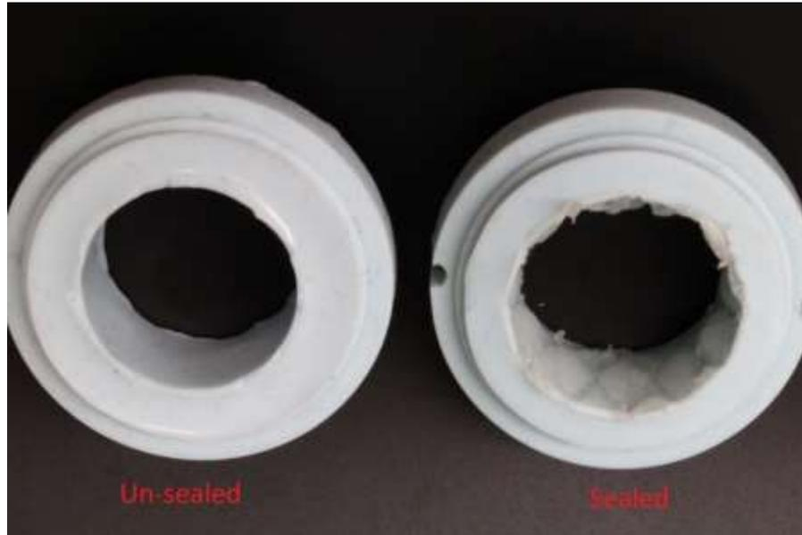
*Fixtures intended to test for total leakage (left) and transvalvular leakage only (right).*
