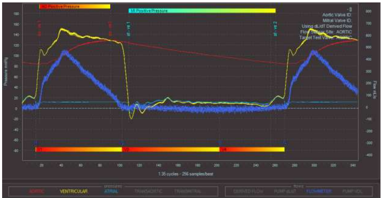
Noise from an improperly grounded flow meter (blue).
